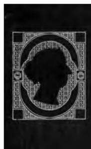
A simulated roller proof *printed intaglio*. The white areas are raised above the surrounding area of the roller and the parts of the image printed black.
