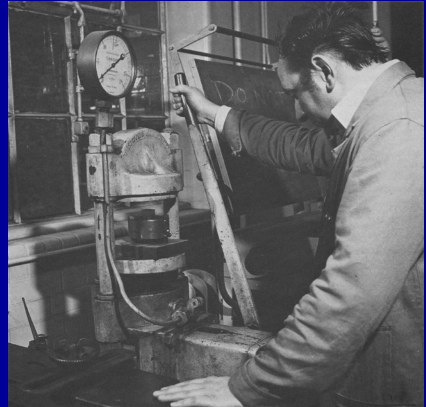
The collar is placed in the hydraulic press which forces the plunger down impressing the die pattern into the lead
