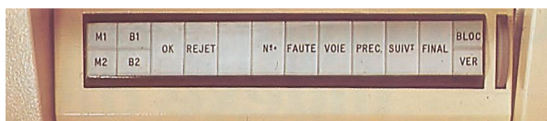
Visual display unit on a poste d'indexation mixte. The computer illuminates the appropriate command when requesting the input of supplementary data from the operator.
